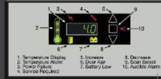
IntrLogic control panel is standard on Revco refrigerators and freezers (except BOD models).
