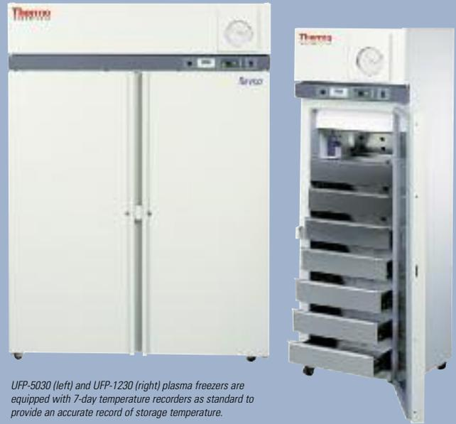
UFP-5030 (left) and UFP-1230 (right) plasma freezers are equipped with 7-day temperature recorders as standard to provide an accurate record of storage temperature.
